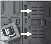
2 2.5-inch storage device installations located on the motherboard tray
