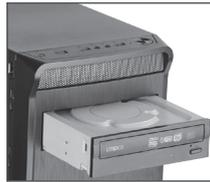
Then insert the optical drive in the designated section as shown in the picture above.
