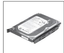
Then insert the clips into the openings on both sides of the drive.
