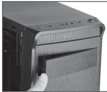
To remove the optical drive cover, first push it outwards from the back and remove it.
