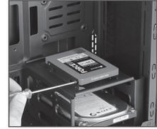
Then with two screws Insert into the desired compartment
