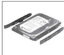
Clips as in the picture above Place on both sides of the desired drive
