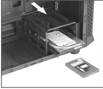
For the installation of the storage device, inside the compartment, where the 2.5-inch drive will be installed.
