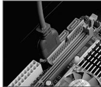
Connect the connector to the socket as shown in the picture above. Make the 20-pin connection to the motherboard.
