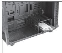
As shown in the picture above, you can select the desired insert the drive into one of the two available slots.
