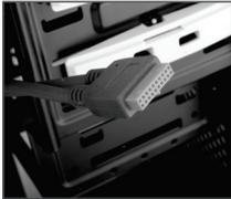
USB 3.0 port on the front panel a 20-pin connector to the motherboard connects through
