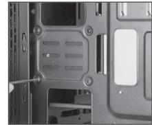
Then secure it to the tray using four screws from the back of the case.
