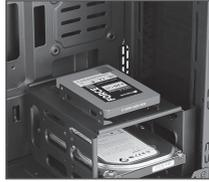
First, place the desired device at the top of the compartment as shown in the illustration.
