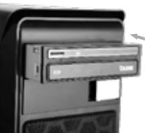
Then insert the optical drive into the designated bay as shown in the picture above.
