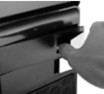
Firstly, pull the clip on the optical drive cover outwards and close it, then disconnect the relevant connections.
