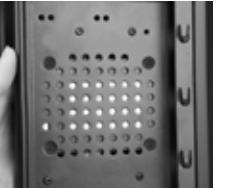
Next, connect the hard drive using 4 special screws.
