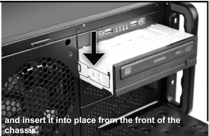
**and insert it into place from the front of the chassis.**
