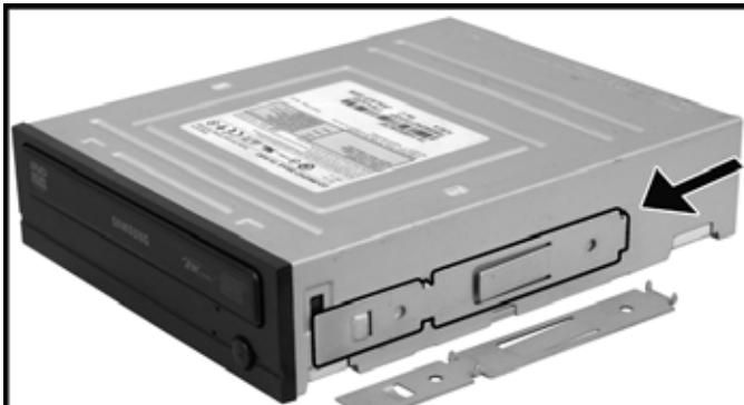
**Mount the metal plate on both sides of the optical drive.**
