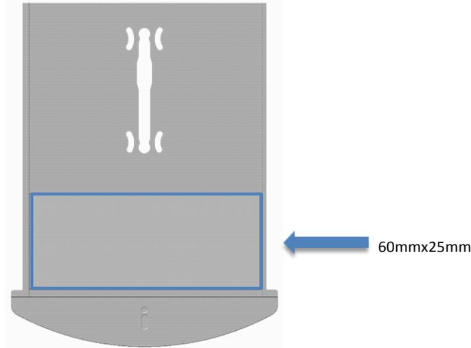
Figure 14. Pull-out Tag Label Emboss Dimensions
