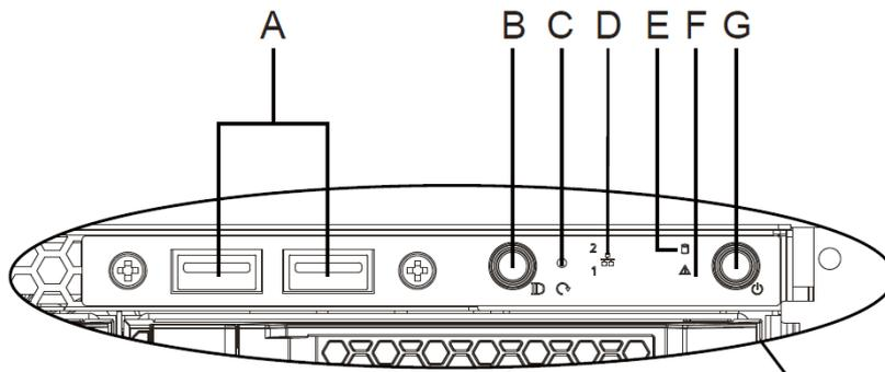
Figure 8. Front Control Panel
