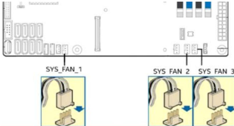
Figure 22. System Fan Connector Locations on Server Board
