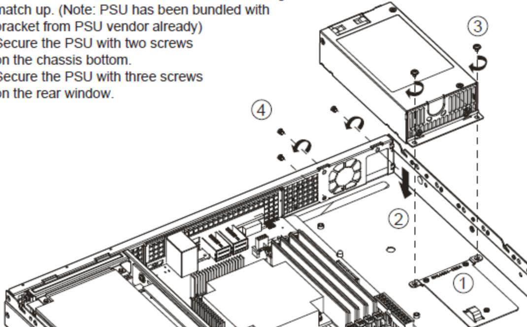
Figure 16. Power Supply installation
