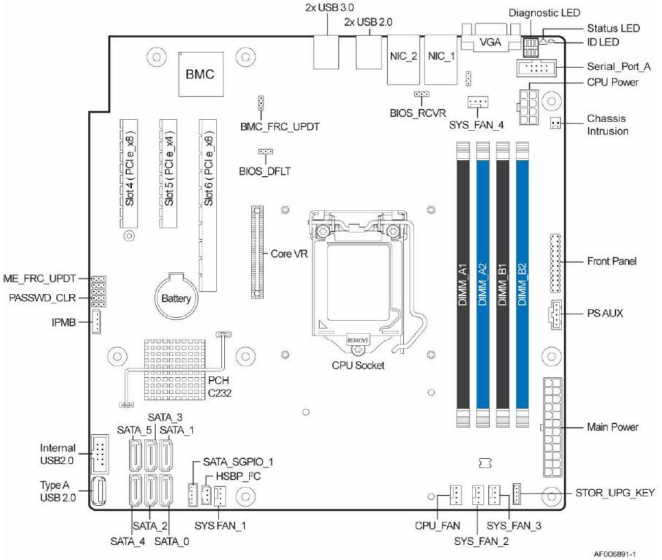
**Figure 4. Server Board S1200SPS Features**
