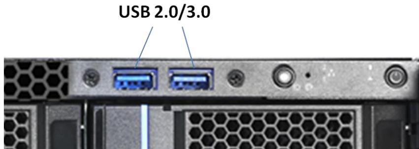
**Figure 38. Front I/O Panel Features**
