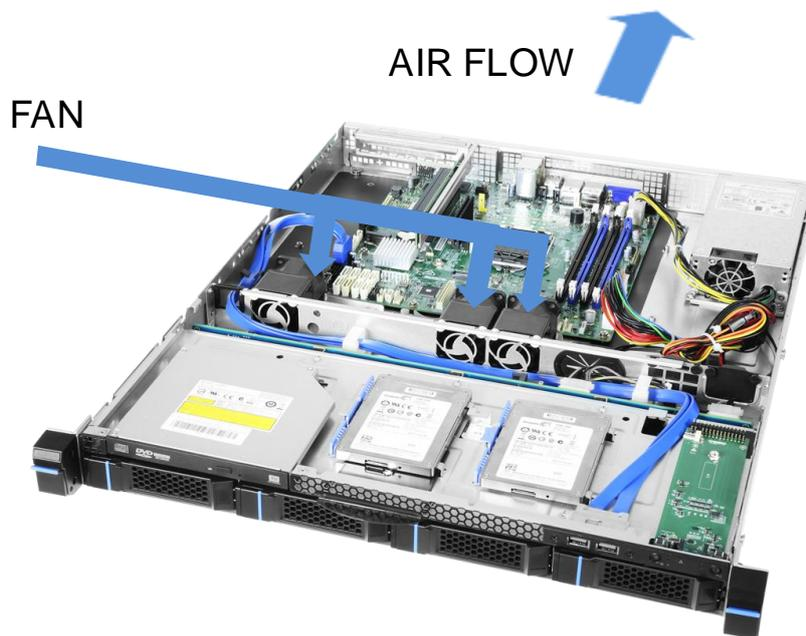
**Figure 19. System Air Flow and Fan Identification**
