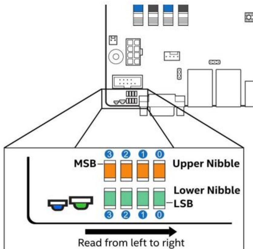
**Figure 46. POST Diagnostic LED Location**
