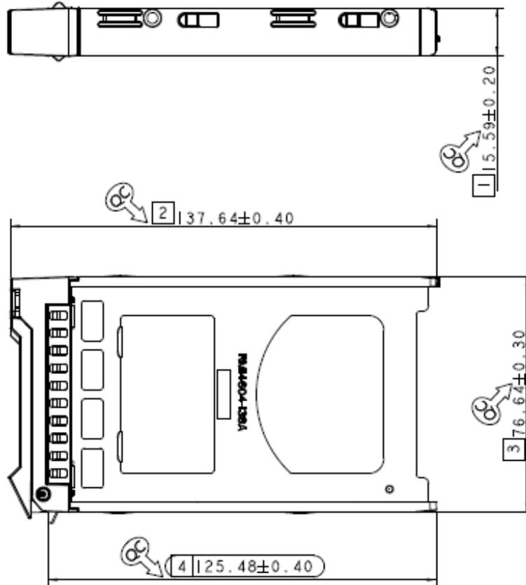
Figure 12. 3.5" HDD Tray Dimensions
