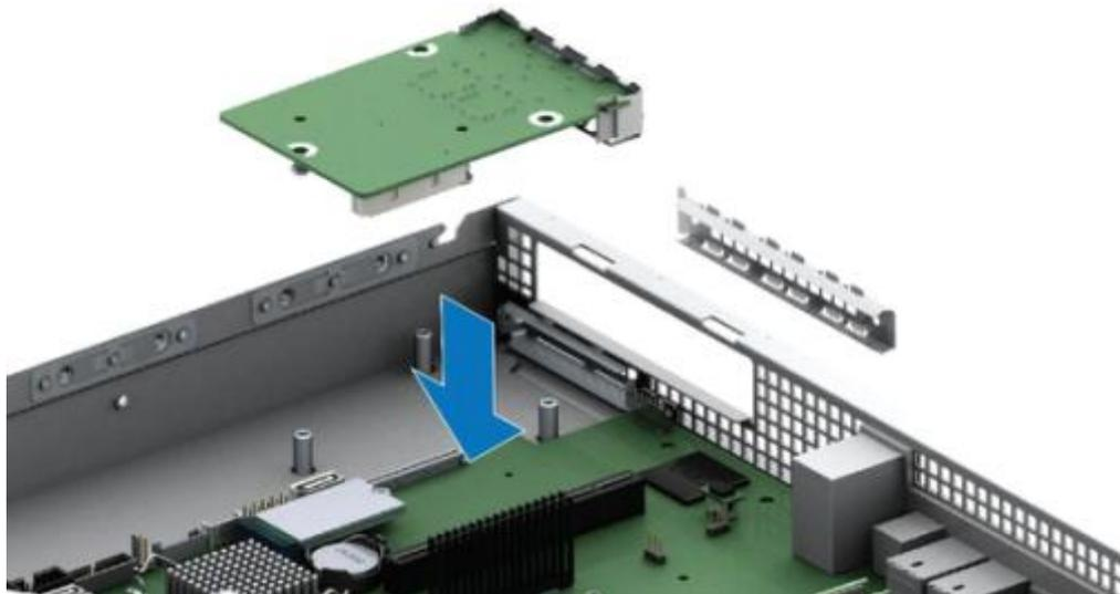
**Figure 43. Intel® I/O Module Placement**
