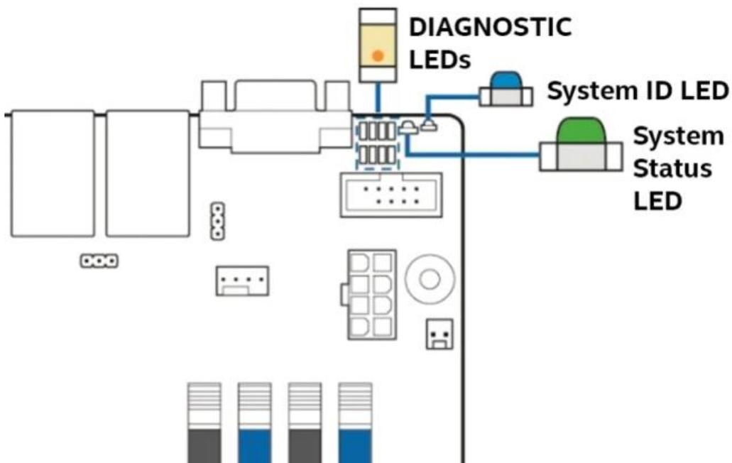
**Figure 5. On-board Diagnostic LEDs**
