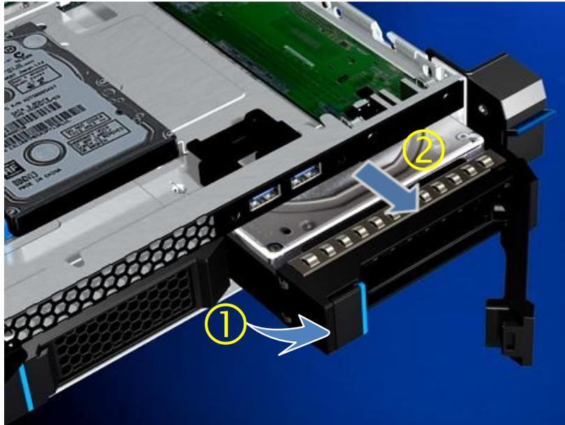
**Figure 25. Hot Swap Storage Device Carrier Removal**
