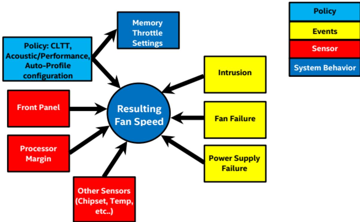
Figure 20.Fan Control Model
