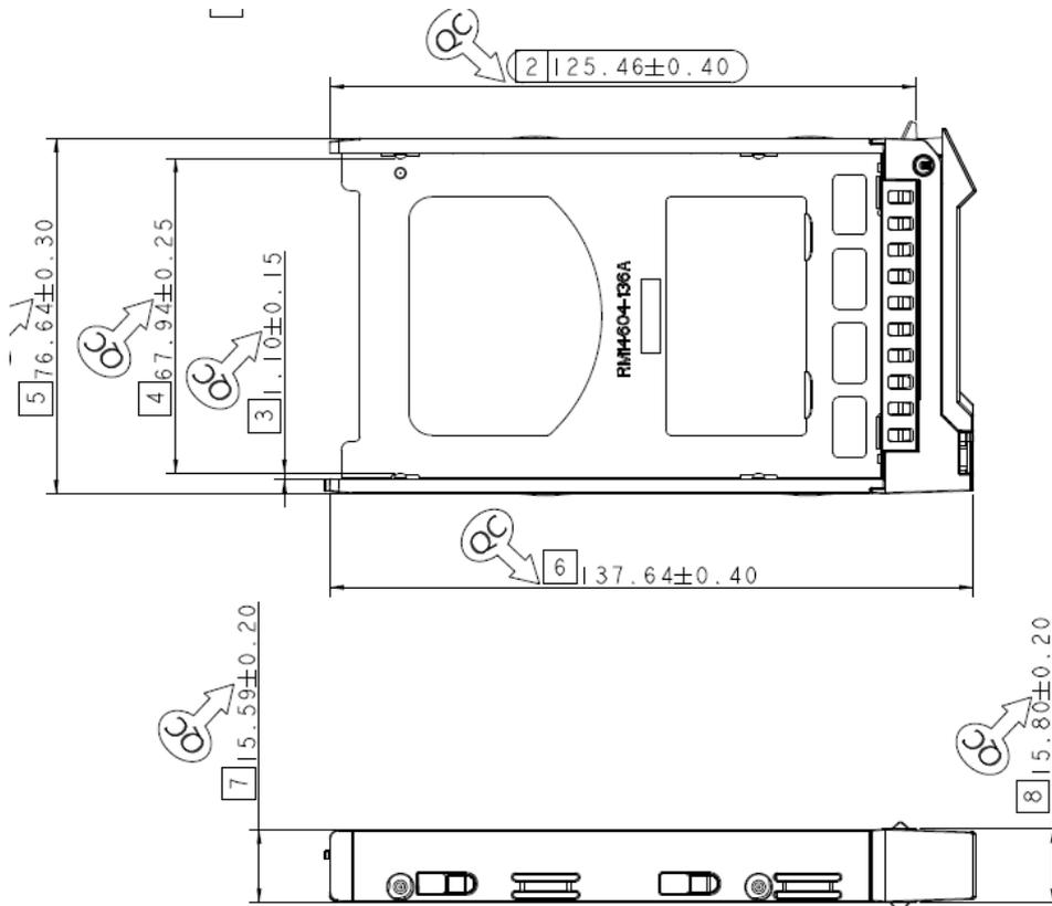
Figure 13. 2.5" HDD Tray Dimensions
