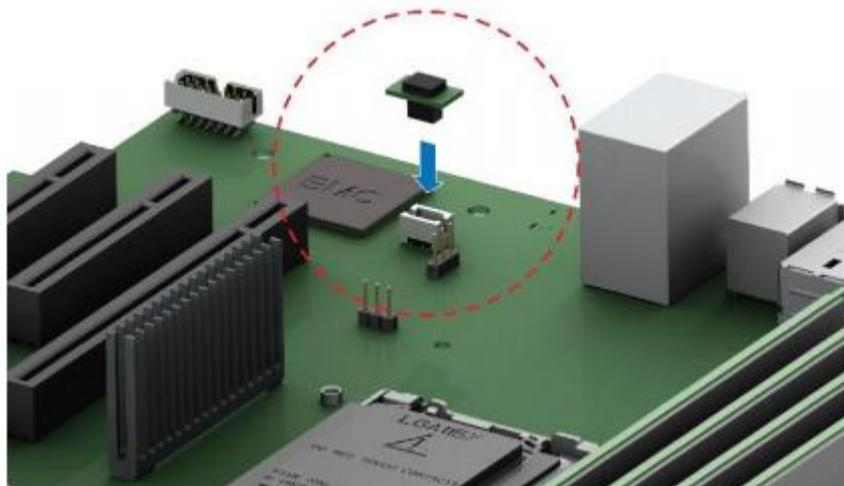
**Figure 44. Intel® RMM4 Lite Activation Key Installation**
