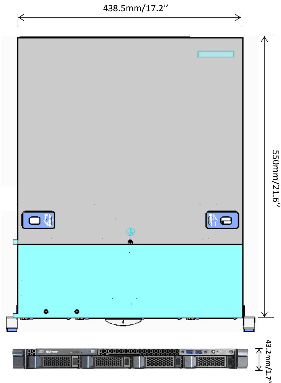
Figure 11. Chassis Dimensions
