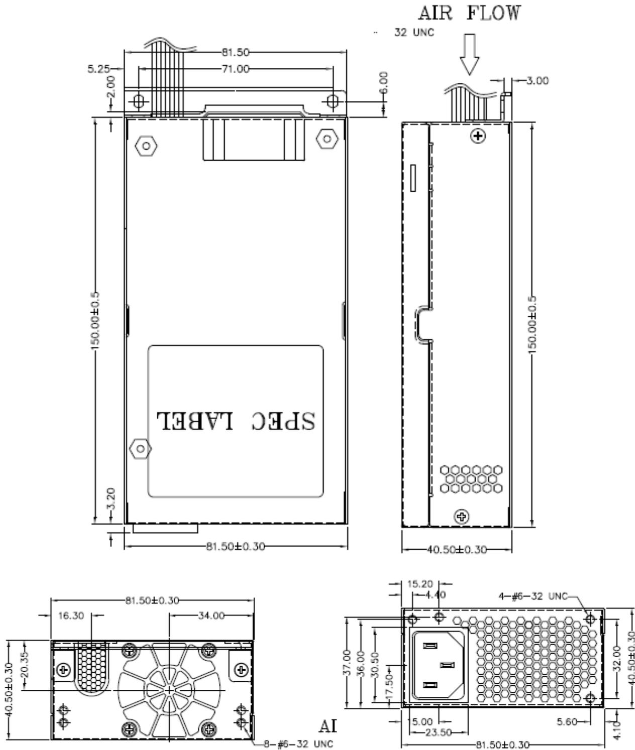
Figure 17. 400W Power Supply Mechanical drawings
