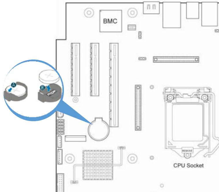
**Figure 45. Replacing the Backup Battery**
